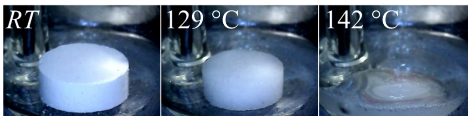
Figure 1. Temperature programmed photographic analysis of Li_2B_{12}H_{12} \cdot xACN showing melting at low temperature.
